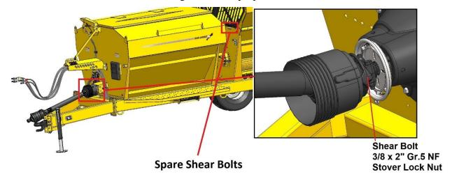
If your shear bolt is shearing excessively, you may be over-loading the machine. If this occurs raise the grate assembly to make the machine less aggressive, or roll the bale more slowly. Always ensure that your machine is running at 1000 PTO RPM.
