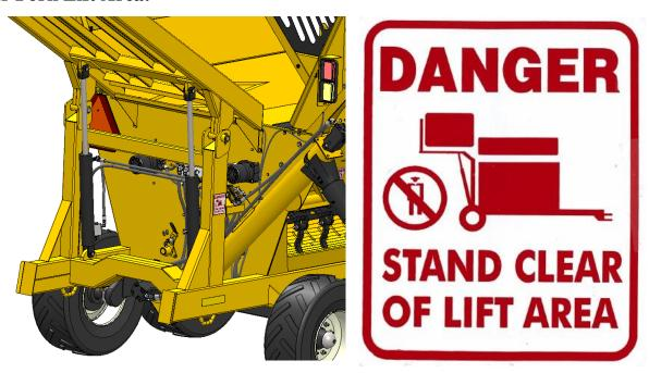
DANGER: Stand clear of lift area. Do not stand under the forks if tractor is running or if bale is resting on forks. Automatic hydraulic safety locks are installed.
