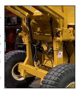
NOTE: Always cover exposed cylinder shafts with grease to avoid rusting of shafts if the unit is not used for extended periods of time. Rusted cylinder shafts are NOT covered by warranty
