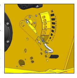
When there is a bale in the tub, the bale's weight will be placed on the hoop grates, making adjustment more difficult. Adjust the machine when it is empty when possible.
