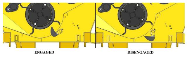
The fine chop adjustment handle is located at the rear of the processor, on the bottom left corner of the tub panel.
