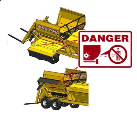
DANGER: Do not stand on the discharge side of the machine while it is in operation.
