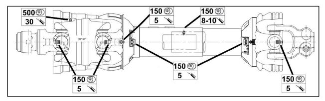
**After storage** for long periods of time, lubricate and check the function of every driveline component before operating. Failure to grease all the joints will **VOID** warranty.
