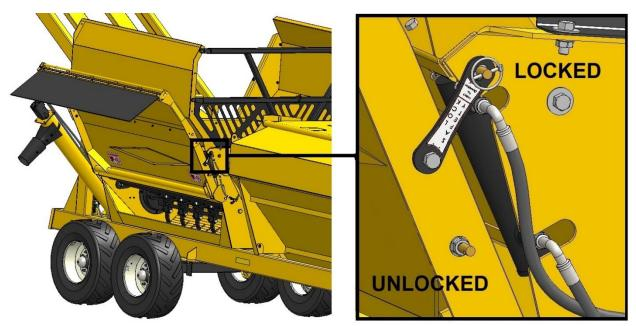
Unlock for operation, Lock for transport and storage
