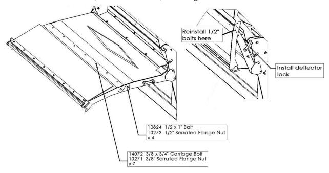
BE CAREFUL WHEN LIFTING THE DEFLECTOR WITH THE OUTER PANEL ABLE TO PIVOT TO AVOID CONTACTING THE TIRES.
