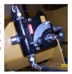
If the operator wishes to feed at a certain feed rate the auger speed can be adjusted to come reasonably close to the desired rate. The operator must first measure the discharge volume or weight per unit of time. This can be done by running the tractor at bale processing engine speed (1000 PTO RPM) and timing how long it takes to fill a small container or pail full of grain. The grain is then either weighed or measured for volume.
