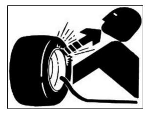
Note: When inflating tires, use a clip-on chuck and extension hose long enough to allow you to stand to one side and NOT in front of or over the tire assembly.
