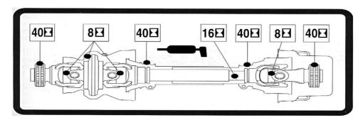
**After Storage** for long periods of time, lubricate and check the function of every driveline component before operating.
