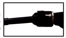
If your shear-bolt is shearing excessively you may be over-loading the machine. If this occurs raise the grate assembly to make the machine less aggressive. Also roll the bale more slowly. Always ensure that your machine is running at 1000 PTO RPM.
