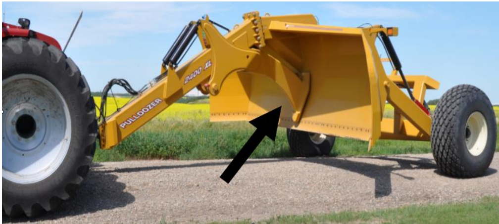
Figure: Trencher in retracted position
