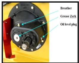
If the gearbox is removed to replace the rotor or perform any other service, add **80 pumps** of grease to the grease zerk upon reinstallation.
