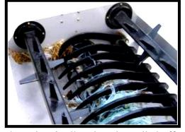
An electric device is also available from suppliers to melt the twine & allow it to be pulled off. Once melted, the twine should be removed immediately to prevent damage to the rotor. It is **NOT PERMITTED** to leave the twine burning on the rotor as this has several adverse effects:
