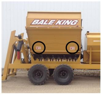
DANGER: Do not stand on the discharge side of the machine while it is in operation.
