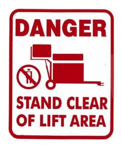
DANGER: Stand clear of lift area. Do not stand under the forks unless safety locks are installed.
