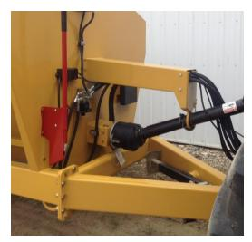
shield. This can be done by loosing the bolt on top of the plastic hose clamp, then pushing or pulling on the hoses to adjust the length.
