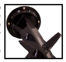
**WARNING**: Before attempting the removal of twine from the rotor, be sure that the machine is stopped and the tractor is shut **OFF**. Place the tractor in park. Twines can be removed with the use of the supplied knife, or any other knife.
