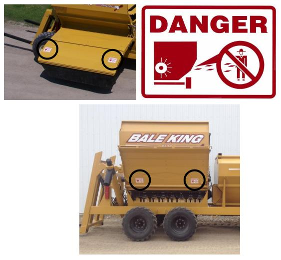
**DANGER:** Do not stand on the discharge side of the machine while it is in operation.
