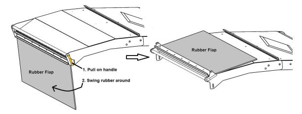
Moving the deflector to the **down** position and flipping the rubber down (above left) will allow the hay to be laid in a windrow, or bunk feeder. Swinging the deflector **up** will allow you to spread straw out over a large area. If you also flip the rubber up (above right), you will be able to "fine tune" the discharge, to control the height and distance.
