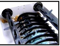
An electric device is also available from suppliers to melt the twine & allow it to be pulled off. Once melted, the twine should be removed immediately to prevent damage to the rotor. It is **NOT PERMITTED** to leave the twine burning on the rotor as this has several adverse effects:
