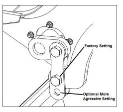
**NOTE:** Upper grate position should be approximately 1/4" flail recession. Lower grate position should allow 1-1/2" flail protrusion. Contact your Bale King dealer if this can't be achieved.
