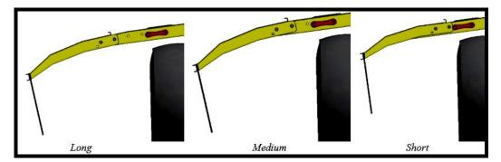
NOTE: Use only the medium and short settings unless required due to tractor width.
