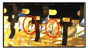
There are two settings for the fine chop, depending on how fine you wish to cut the material. These settings are achieved by pulling the handle towards the back of the machine, then selecting the desired hole.
