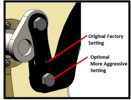
**NOTE:** Upper grate position should be approximately 1/4" flail recession. Lower grate position should allow 1-1/2" flail protrusion. Contact your Bale King dealer if this cannot be achieved.
