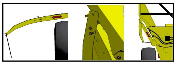
Be sure that the outer deflector fits nicely outside the tub walls. Some fine tuning may be required. Replace the bolts on the front and back in the available holes as shown. The deflector should now fit inside the width of the wings.
