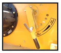
• **Position #6:** Lowest grate position, most aggressive fastest rate of feed.
