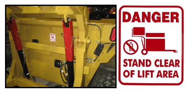
**DANGER:** Stand clear of lift area. Do not stand under the forks unless safety locks are installed.
