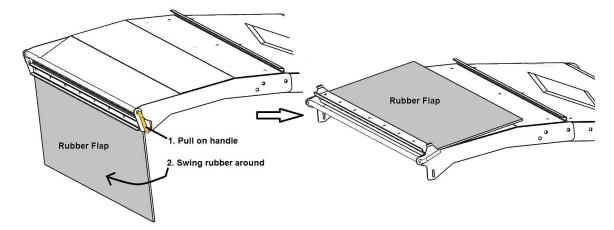
Moving the deflector to the **down** position and flipping the rubber down (above left) will allow the hay to be laid in a windrow, or bunk feeder. Swinging the deflector **up** will allow you to spread straw out over a large area. If you also flip the rubber up (above right), you will be able to "fine tune" the discharge, to control the height and distance.
