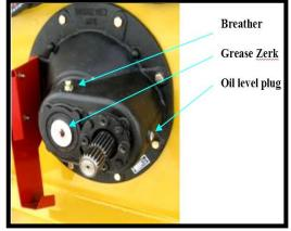
The gear box requires GL5 80W90 gear oil. The oil should be filled to the level plug and checked on a regular basis.
