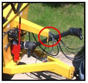
The hydraulic hoses may need to be adjusted to best fit your tractor, to avoid damage from rubbing on the PTO shaft shield. This can be done by loosing the bolt on top of the plastic hose clamp, then pushing or pulling on the hoses to adjust the length, and retightening the bolt.
