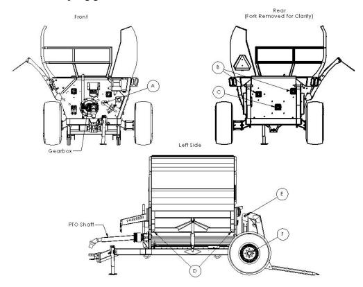
The gear box requires GL5 80W90 gear oil. The oil should be filled to the level plug (approximately **500 mL**). Ensure the breather is installed and free of obstruction.
