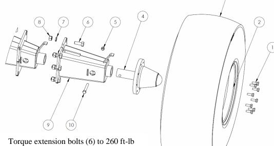
Torque extension bolts (6) to 260 ft-lb Torque spindle bolt (10) to 115 ft-lb Torque wheel studs (1) to 125 ft-lb
