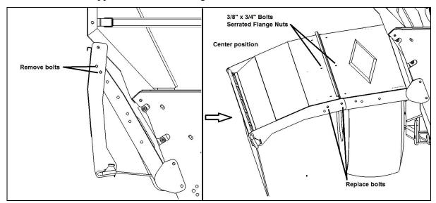
WARNING: Do not swing the deflector down before the deflector is unfolded. It will hit the tire.
