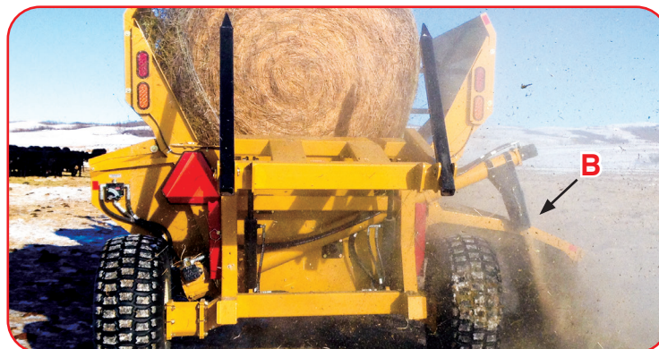
Model 5300: Process any round bale. Comes with twin agitator feeding system. Shown with available 3rd bale clamping system.
