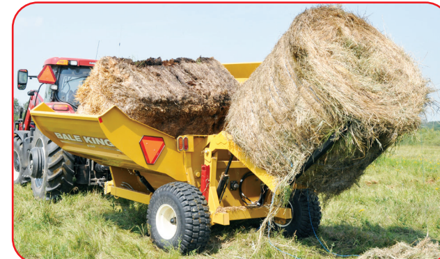
Model 8200: Process square or round bales. The twin agitator system provides grip on both sides of the rotor to manipulate square bales.
