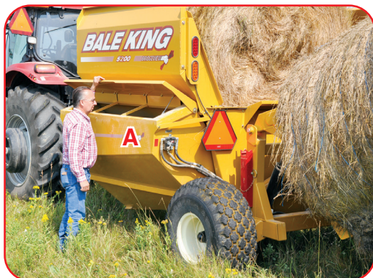
TR Total Ration: This bolt on kit comes with a 40 bu. hopper (A) and hydraulically driven discharge auger (B). Process any round bale and
