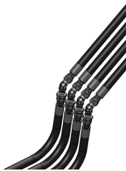
Figure 21 - Hitch to tractor hose connection
