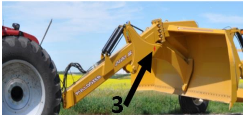
Figure 1.2.1: Shows the safety locks marked by arrows
