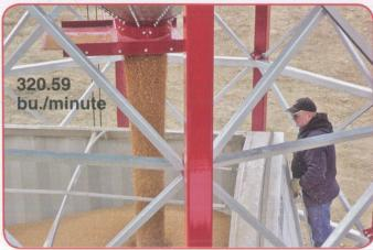
With a gravity flow rate of 320.59 bu./minute you can fill a semi in about 3 minutes.
