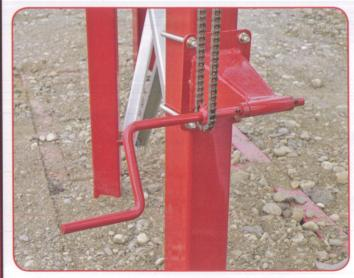
Ground level chute control. Can be set on your concrete pad or the available steel foundation.
