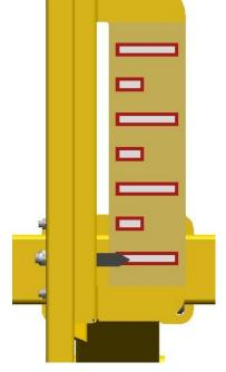
An indicator is provided to show you how wide the rear end is set. This will allow you to consistently set the machine to your desired windrow width. The needle moves up to indicate a wider windrow, while the bottom position indicates transport width.
