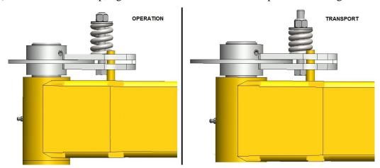
IMPORTANT: Ensure that the spring is loosened back off before operation or the rake will be very difficult to turn or back up.
