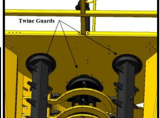
also help keep twines away from the wheel bearing seal. Remove twine any time you notice it on the axle.
