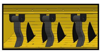
It is recommended that the knives be lowered when bedding straw as it will affect your spread pattern. Adjust the machine as needed. There are two engaged settings for the fine chop, depending on how fine you wish to cut the material. These settings are made using the handle in the front bottom right corner.
