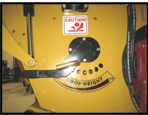
The Bale King should be adjusted according to various bale conditions to achieve a rate of feed of approximately 1.5 to 2 minutes\*. Light brittle material such as wheat straw may allow faster processing while tough stringy material such as slough hay, green feed, or flax will require slower processing. Hoop grate adjustment should be checked periodically.
