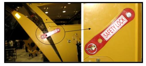
Deflector Safety Lock: Unlock for Operation, Lock for Transport and Storage
