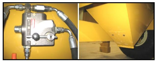
A door is provided at the bottom of the tank for clean out if required.
