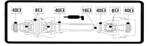
After Storage for long periods of time, lubricate and check the function of every driveline component before operating.
