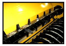
It may be necessary to change direction of the bale when loose debris builds on either side of the bale chamber. This will remove the loose debris preventing spillage from the machine.
