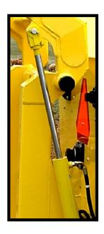
NOTE: Always cover exposed cylinder shafts with grease to avoid rusting on shafts if unit is not used for extended periods of time. Rusted Cylinder shafts are not covered by warranty.
