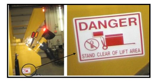
Danger: Stand clear of lift area; do not walk under forks unless safety locks are installed
