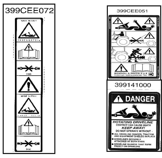
Do not operate the machine without all driveline, tractor, and implement shields in place. Drive-line shields must turn freely on the driveshaft.
