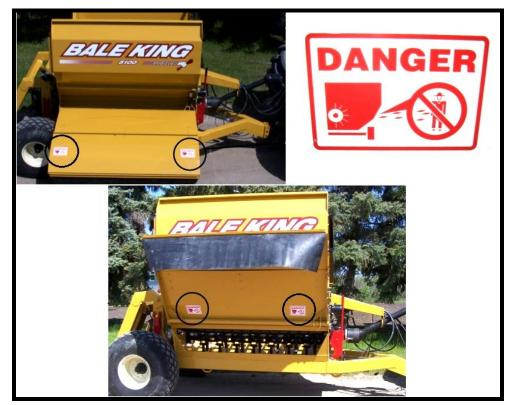
**DANGER:** Do not stand on the discharge side of the machine while it is in operation.
