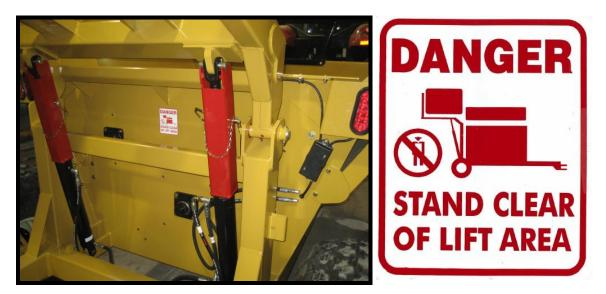
DANGER: Stand clear of lift area. Do not stand under the forks unless safety locks are installed.
