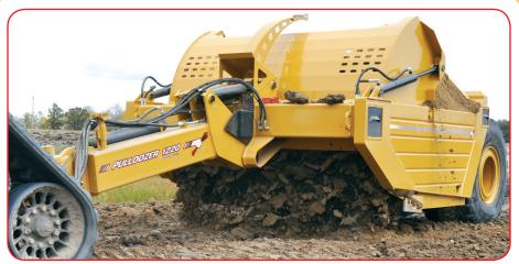
Better performance in tough conditions: Extra-large apron opening ensures smooth unloading in tough conditions. Push-off gate travels slightly past the cutting blade for total cleanout.
